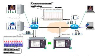
Fig. 1 Real-time burst measurement using MD1230B
