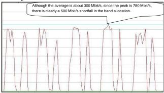
Fig. 2 Monitored VoD Server Stream
